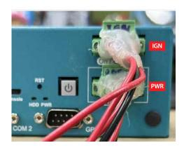
For testing purpose, you can refer to the picture blow to simulate ignition signal input controlled by a latching switch.
