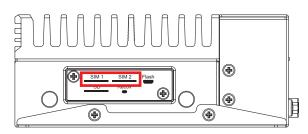
The external Nano SIM card offers wireless communication capability by M.2 key B 4G/5G Card to the system.
