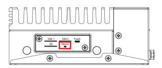
Press the Button enter Force Recovery Mode. Button is held down while either system is first powered on, or by pressing & releasing reset button while Recovery button is pressed.
