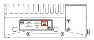
The EAC-6000 USB Recovery mode provides an alternate boot device (USB). In this mode, the system is connected to a host system and boots over USB. This is used when a new image needs to be flashed. USB0 must be available to use as USB Device for USB Recovery Mode.
