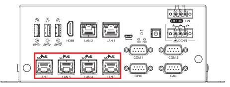
There are 4 RJ45 connectors in the front side of EAC-6200. It supports IEEE802.3at (PoE+) Power over Ethernet (PoE) connection delivering up to 25W/54V per port and 1000BASE-T gigabit data signals over standard Ethernet Cat 5/Cat6 cable.
