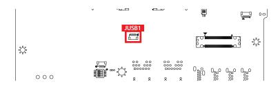
The USB Connector is reserve for GPS function. The USB Bus is switched by software control.
