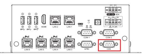
CAN Bus Connector Pin Out:
