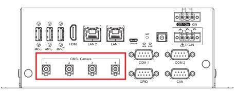
There are four FAKRA connectors in the front side of EAC-6100. Each camera connects to the EAC-6100 through a single coax cable. Using GMSL2 (Gigabit Multimedia Serial Link) connections, the cameras are connected to a two-port deserializer. The output of the deserializer is MIPI CSI-2.
