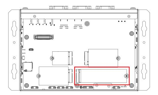
Step 2 Install M.2 Key M cover into slot.
