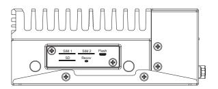
There are some ports SIM1, SIM2, Flash, M-SD Card and Recovery Button are placed on the side panel. It has a case cover these ports.
