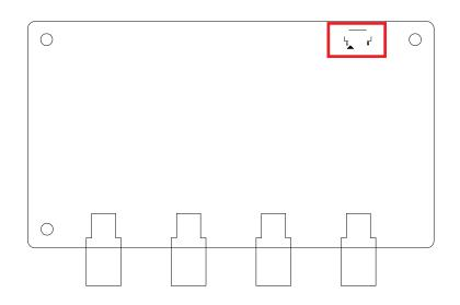
The JMFP Header is connected to the GMSL deserializer FSYNC input. JMFP Header Pin Out:
