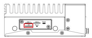
The external Micro SD card provides additional storage expansion. It is located behind the cover-plate on the front panel.
